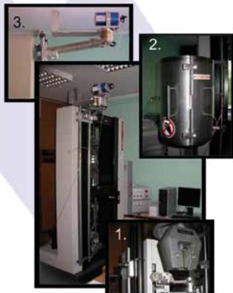
Tensile testing machine INSTRON 6025, improved by Zwick/Roell, load capacity 100 kN
