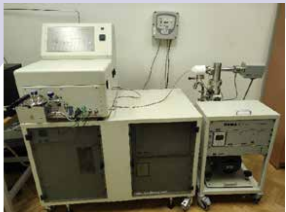
Sievert's apparatus (IMI HTP Hiden Isochema) connected to a mass spectrometer.
