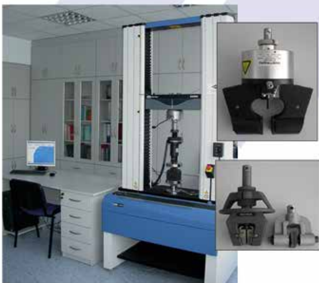
Tensile testing machine INSTRON 3382, load capacity 100 kN
